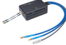
Figure 3. Four remote heads are available for the pattern generator module M8042A. At the top the 120 GBd remote heads M8059A and M8069A are shown with 1.0 mm connectors to accommodate close connection to the device under test for symbol rates up to 120 GBd. The 64 GBd remote heads M8058A and M8068A are shown at the bottom, these provide 1.85 mm connectors. The three cables on the back side of the remote heads are used to connect with the M8042A pattern generator module and are not removable.
