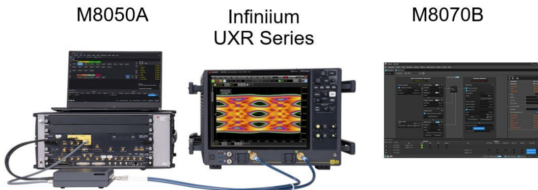
Figure 23. The M8070ADVB controls the UXR and uploads the decoded pattern streams for synchronization and comparison with expected patterns.
