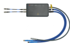
Figure 3. Four remote heads are available for the pattern generator module M8042A. At the top the 120 GBd remote heads M8059A and M8069A are shown with 1.0 mm connectors to accommodate close connection to the device under test for symbol rates up to 120 GBd. The 64 GBd remote heads M8058A and M8068A are shown at the bottom, these provide 1.85 mm connectors. The three cables on the back side of the remote heads are used to connect with the M8042A pattern generator module and are not removable.
