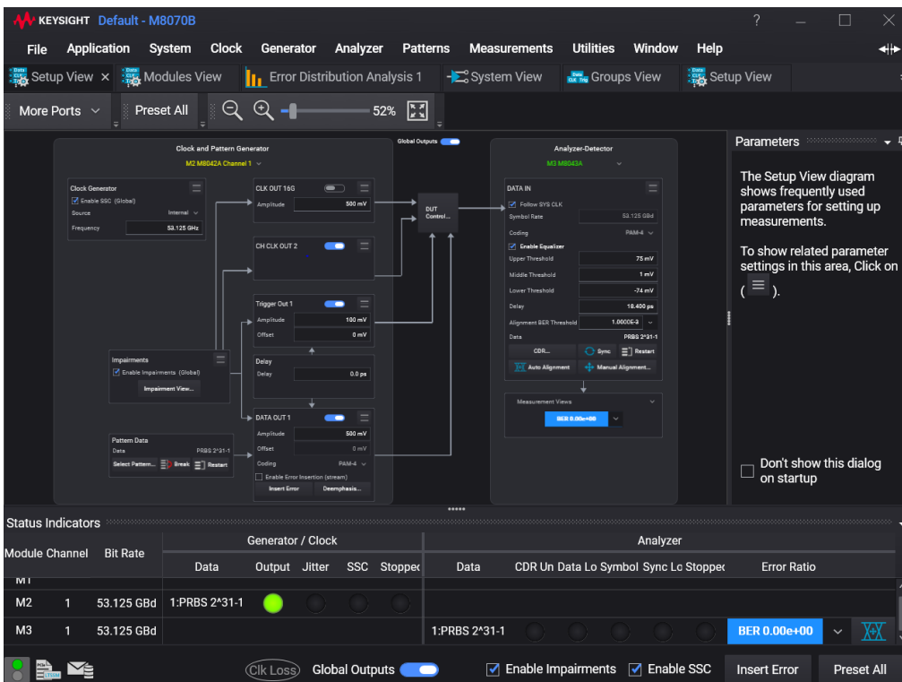
Figure 24. The M8070B system software is required to control the M8050A high-performance BERT. The user interface provides control of all parameters. It provides a graphical user interface and remote control via SCPI. Shown is the setup view with the M8009A clock module, the M8042A pattern generator module, and the M8043A error analyzer module on the right side.
