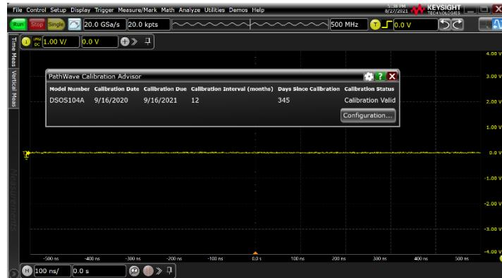
Import your instrument's calibration status document from the main PCA screen. Or, use PCA to access calibration certificates and test reports with a link to the online Keysight Support Portal ([support.keysight.com](http://support.keysight.com)).
