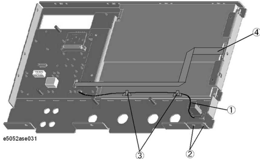
**Table 5-33** Front Assembly (Standby Switch / Cover)
