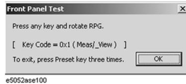
**Step 5.** To exit the front panel test, press **Preset** key three times.
