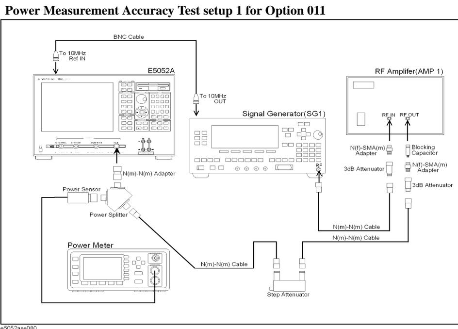
**Step 3.** Press **[Preset] - Factory** to initialize the E5052A, then set the E5052A as follows. In case of installing the firmware revision 1.00/1.10, press **[Preset] - OK**.
