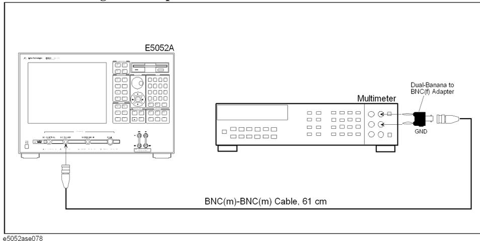
**Step 2.** Press **[Preset] - Factory** to initialize the E5052A, then set the E5052A as follows. In case of installing the firmware revision 1.00/1.10, press **[Preset] - OK**.
