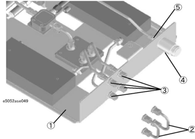
**Table 5-25 Freq/Power Detector Module Attachment Assembly**
