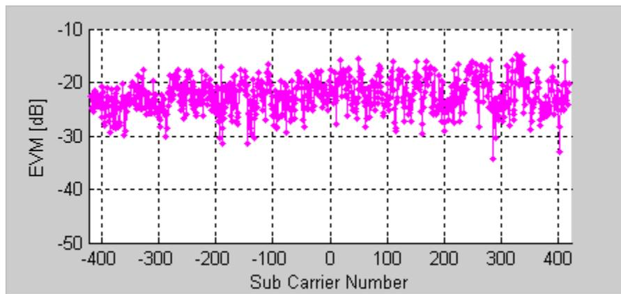
Figure 6-20. IQsignal 802.16e—EVM vs. Carrier Plot
