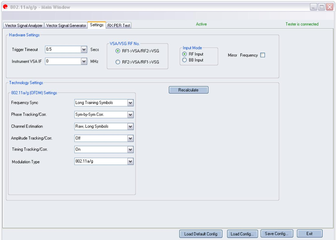
**Figure 4-19. IQsignal 802.11a/g Application—Settings Screen**
