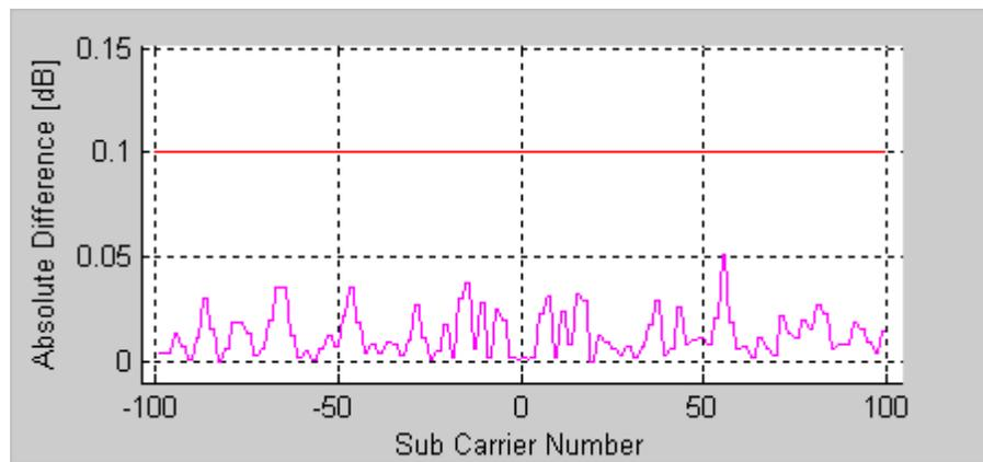
Figure 6-10. IQsignal 802.16d—Spectral Delta Plot
