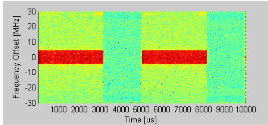
Figure 6-29. IQsignal 802.16e—Spectrogram Plot
