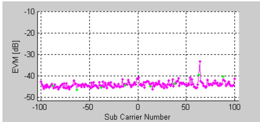
Figure 6-4. IQsignal 802.16d—EVM Plot
