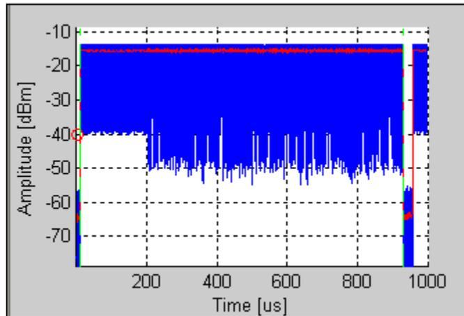
Figure 4-31. IQsignal 802.11b—Amplitude vs. Time
