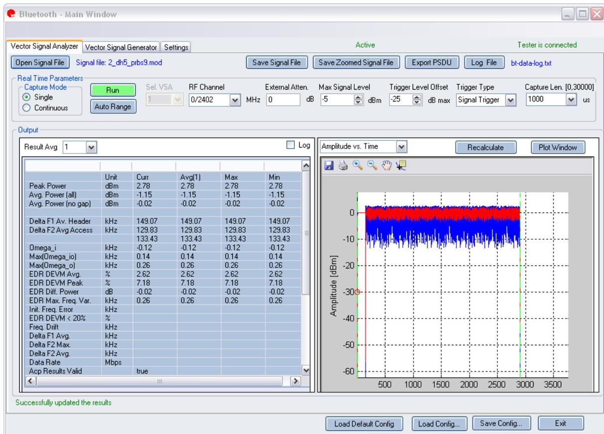
Figure 5-1. IQsignal Bluetooth Application—VSA Screen
