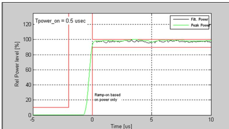
Figure 5-7. IQsignal Bluetooth—Power On Ramp Plot
