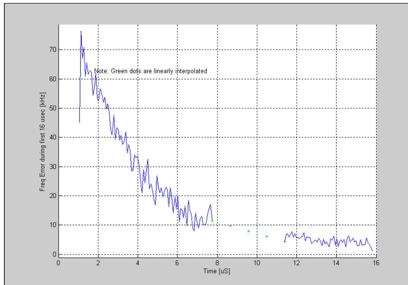
Figure 4-9. IQsignal 802.11a/g—Coarse Frequency Error for Short and Long Training Sequence (OFDM 802.11a/g Signal)
