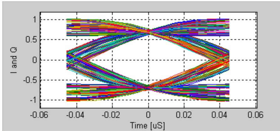
Figure 4-23. IQsignal 802.11b—Eye Diagram Plot
