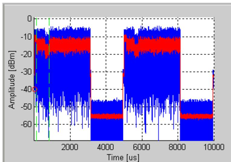
Figure 6-18. IQsignal 802.16e—Amplitude vs. Time Screen
