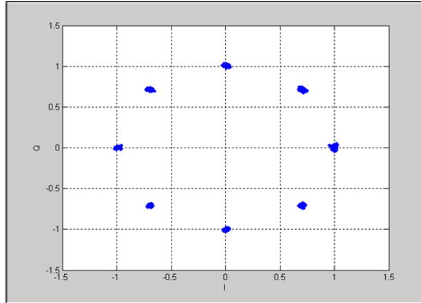
Figure 5-14. IQsignal Bluetooth—Symbol Constellation Plot
