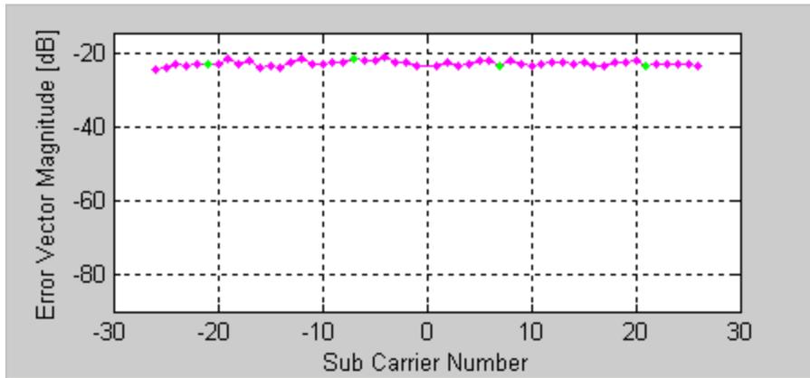
Figure 4-6. IQsignal 802.11a/g—EVM vs. Carrier
