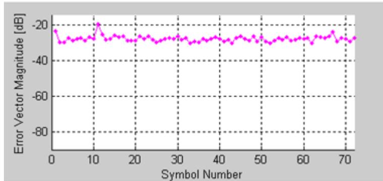
Figure 4-44. IQsignal 802.11n—EVM vs. Time
