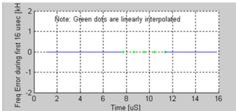
Figure 4-45. IQsignal 802.11n—Frequency Error
