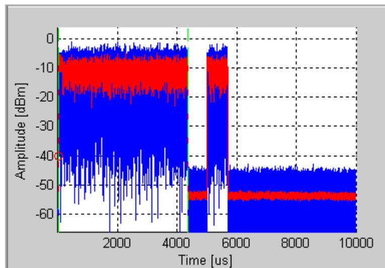
Figure 6-2. IQsignal 802.16d—Amplitude vs. Time Plot
