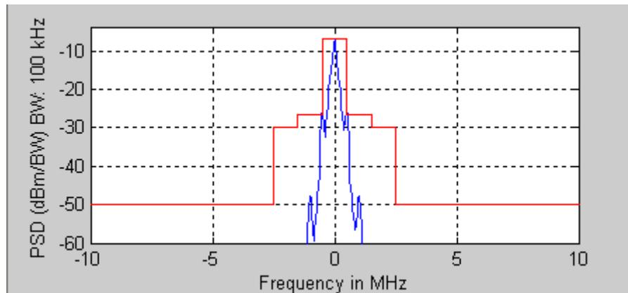
Figure 5-9. IQsignal Bluetooth—Spectrum Mask Plot
