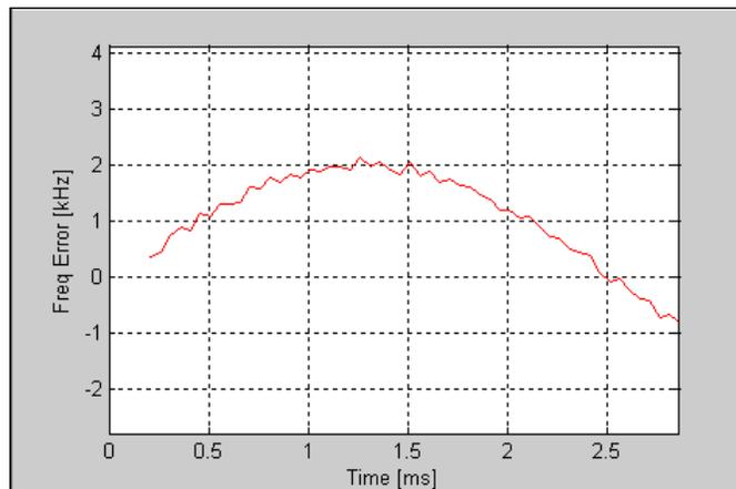
Figure 5-5. IQsignal Bluetooth—Frequency Error Plot
