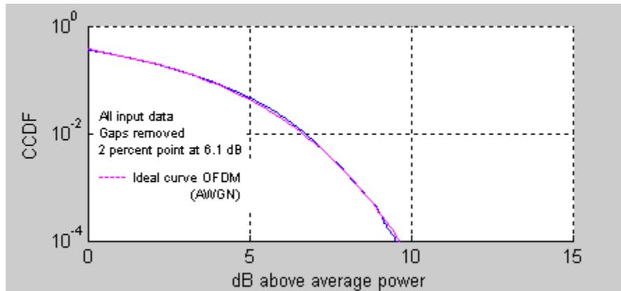
Figure 6-19. IQsignal 802.16e—CCDF OFDM Signal
