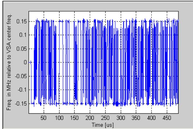
Figure 5-12. IQsignal Bluetooth—FM Demodulator Plot
