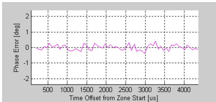
**Figure 6-8. IQsignal 802.16d—Phase Error Plot**
