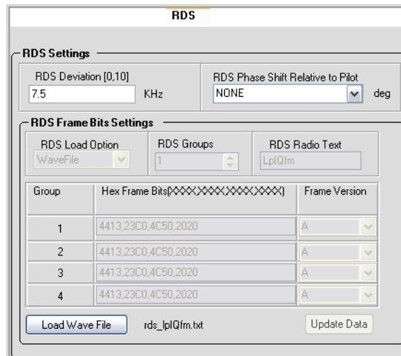
Figure 9-6. IQsignal—RDS Tab
