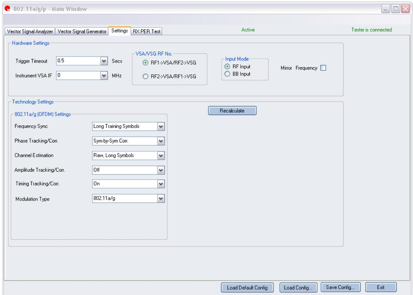
Figure 3-4. IQsignal Application—802.11 a/g/p Settings Screen
