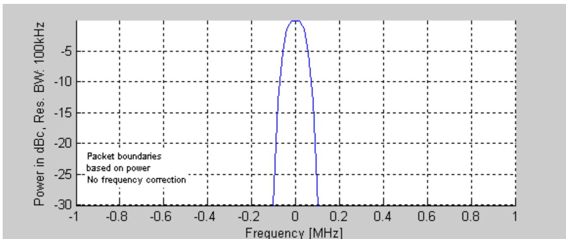
Figure 5-15. IQsignal Bluetooth—LO (DC) Leakage
