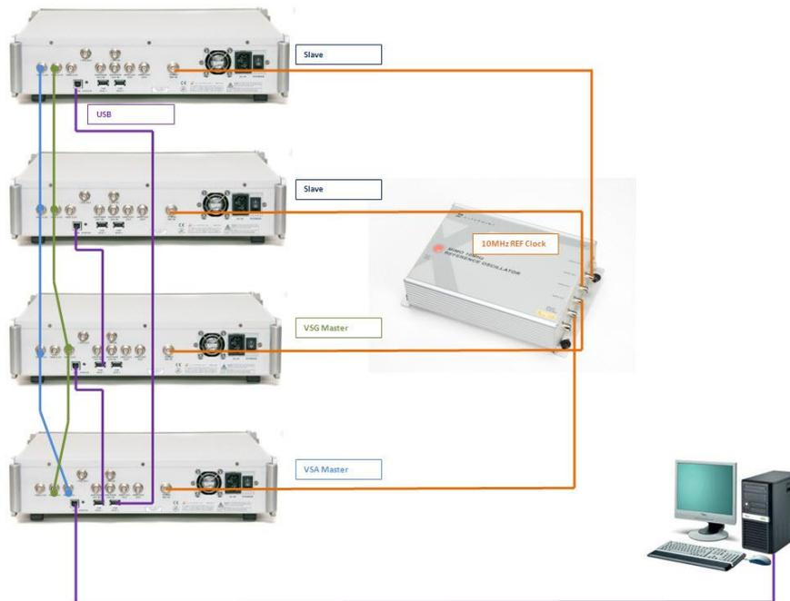
**Figure 1-6. IQ2010 Multiple Tester Setup**
