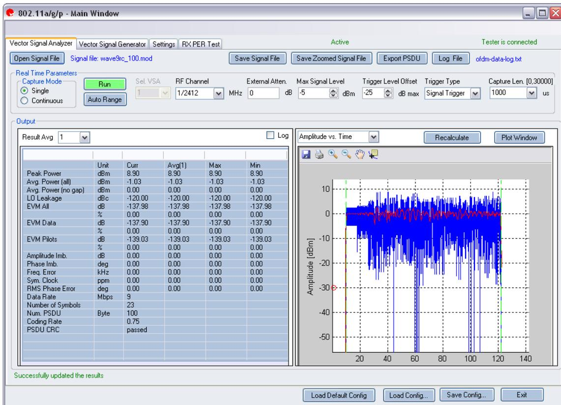
Figure 3-2. IQsignal Application—802.11 a/g/p Vector Signal Analyzer Screen
