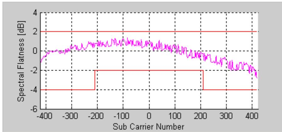
Figure 6-27. IQsignal 802.16e—Spectral Flatness Plot
