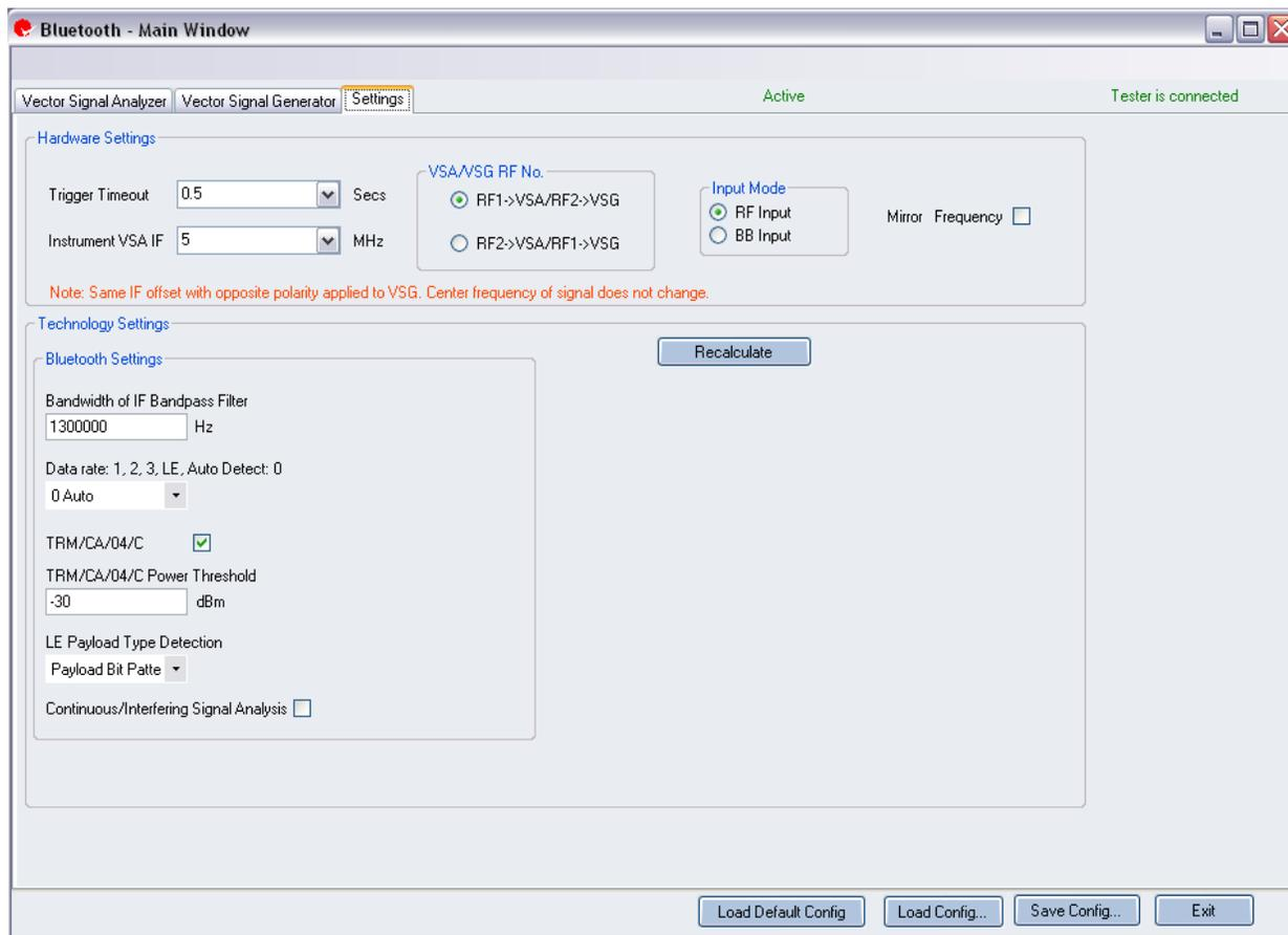
**Figure 5-16. IQsignal Bluetooth Application—Settings Screen**
