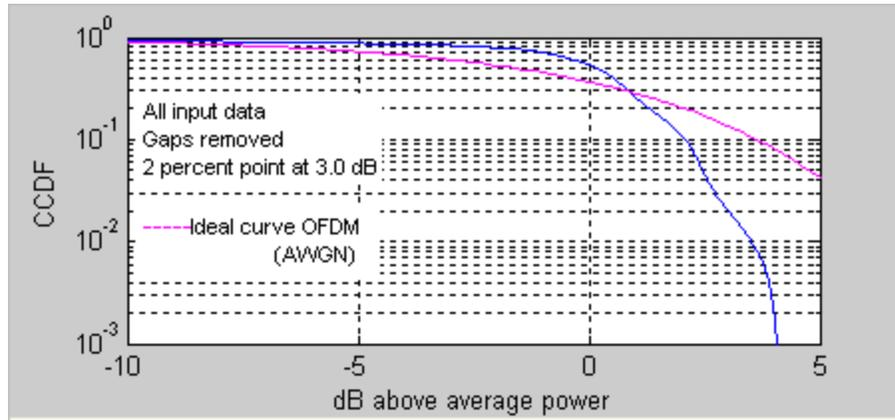
Figure 4-21. IQsignal 802.11b—CCDF OFDM Signal
