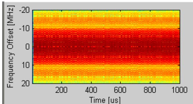
Figure 4-32. IQsignal 802.11b—Spectrogram
