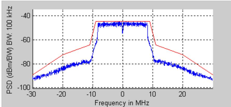
Figure 4-14. IQsignal 802.11a/g—Spectrum Mask Plot
