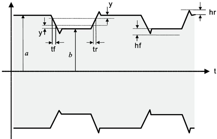
Figure 10-7: Pulse Shape for Manchester Coding at 202kbps and 424kbps [Courtesy of ISO18092 (ECMA340) Specification]
