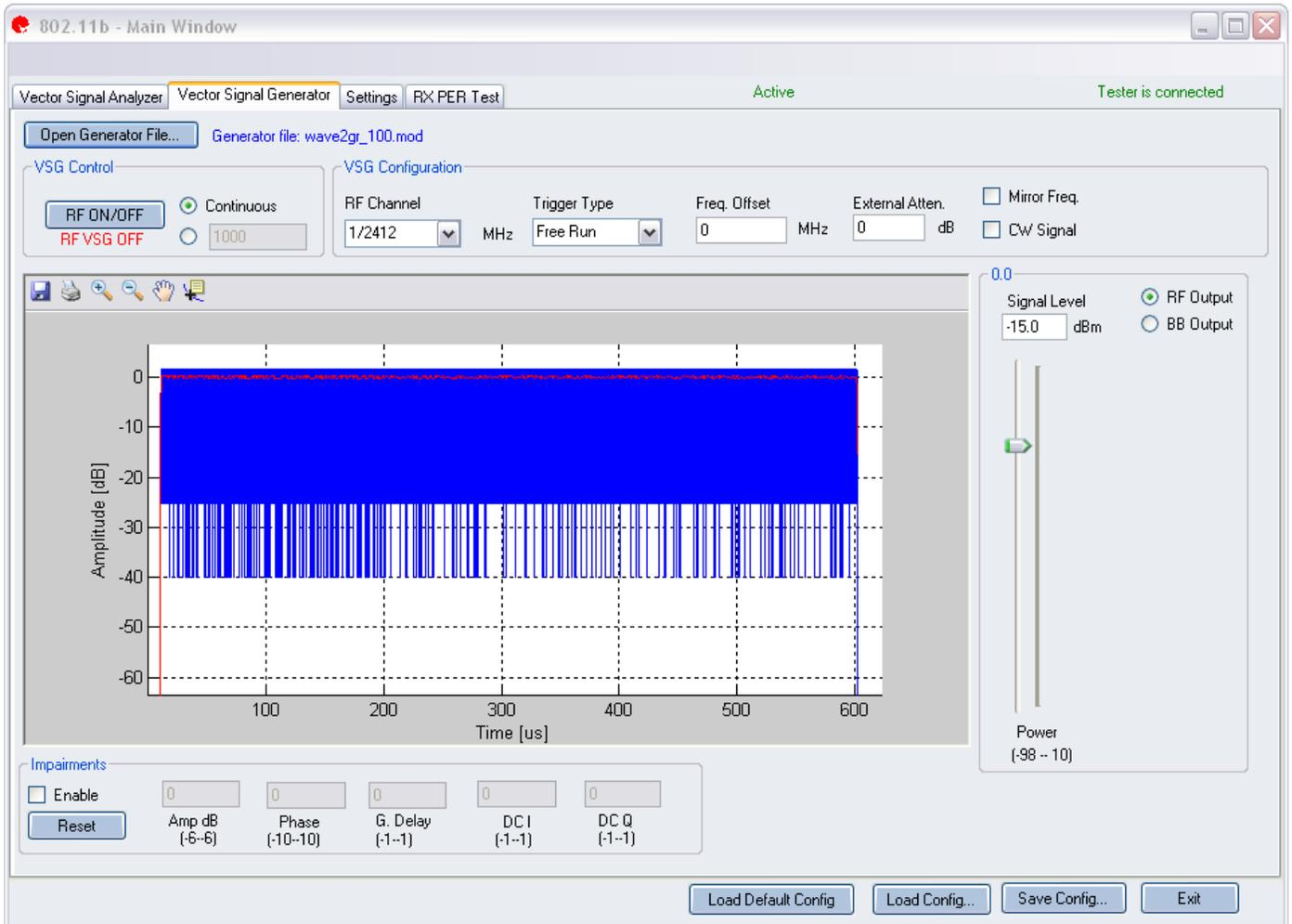
**Figure 4-33. IQsignal 802.11b—VSG Screen**
