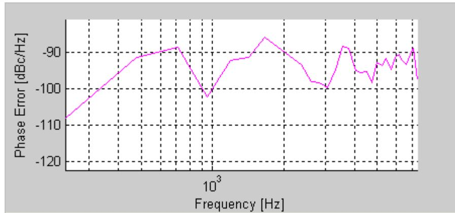
Figure 6-9. IQsignal 802.16d—Phase Error PSD Plot
