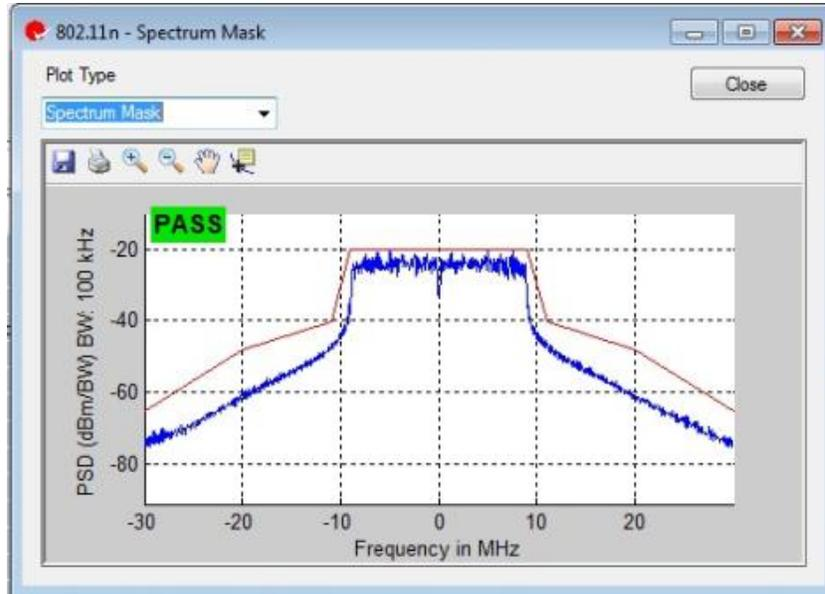
Figure 4-51. IQsignal 802.11n—Spectrum Mask at 60 MHz Frequency
