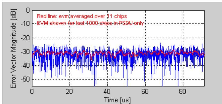
Figure 4-30. IQsignal 802.11b—EVM vs. Symbol Plot
