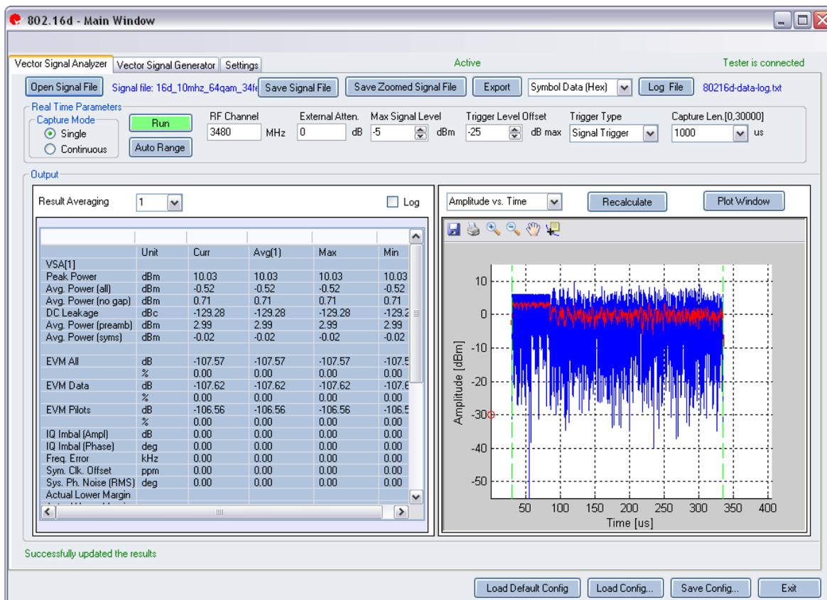
Figure 6-1. IQsignal 802.16d Application—VSA Screen
