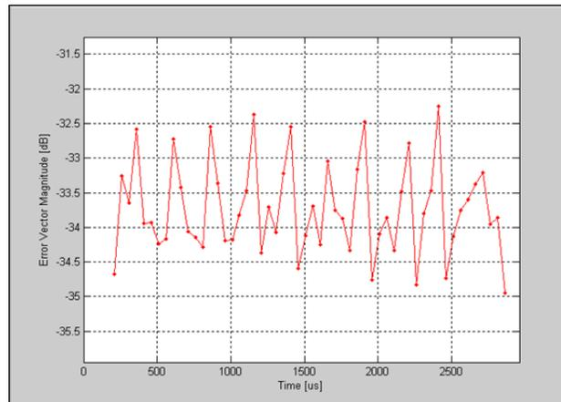
**Figure 5-3. IQsignal Bluetooth—EVM vs. Symbol Plot**
