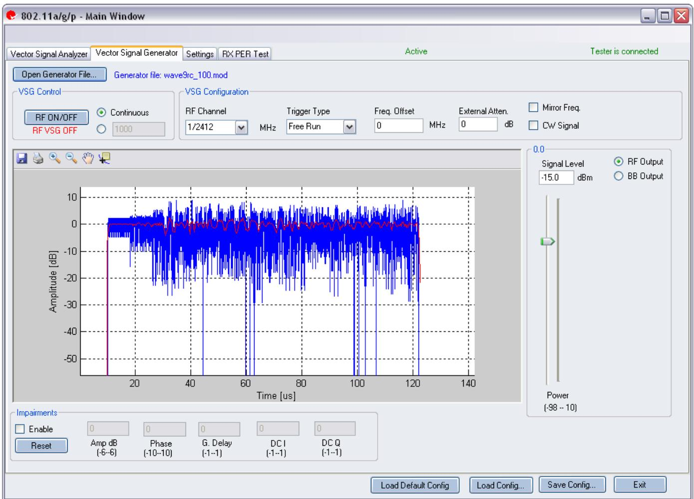
Figure 3-3. IQsignal Application—802.11 a/g/p Vector Signal Generator Screen
