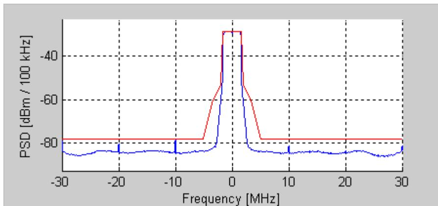
Figure 6-14. IQsignal 802.16d—PSD Plot
