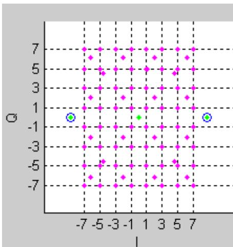
Figure 6-28. IQsignal 802.16e—Symbol Constellation Plot
