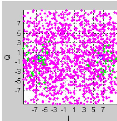
Figure 6-12. IQsignal 802.16d—Symbol Constellation Plot
