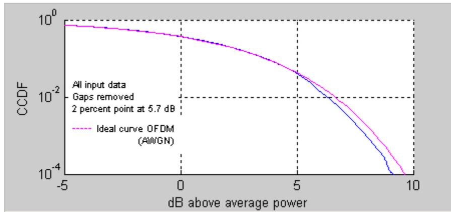
Figure 6-3. IQsignal 802.16d—CCDF OFDM Signal
