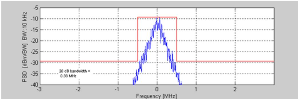
Figure 5-10. IQsignal Bluetooth—20 db Bandwidth Plot
