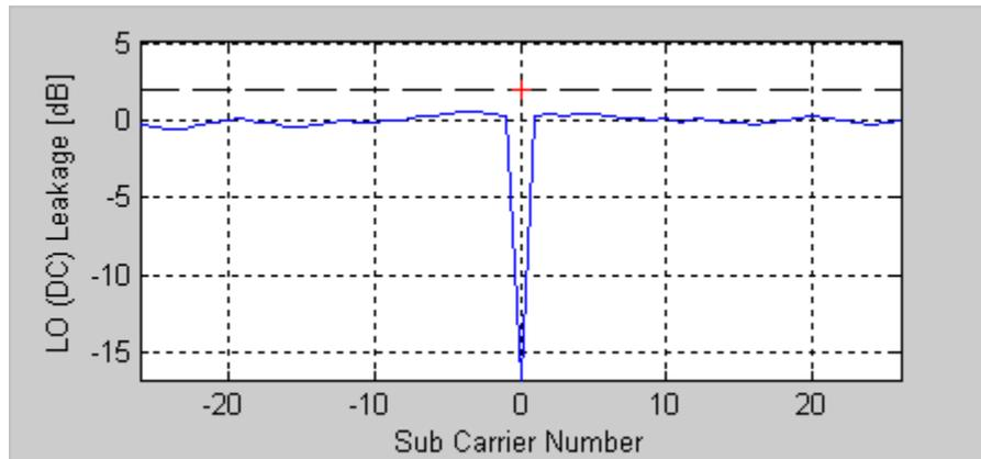
Figure 4-11. IQsignal 802.11a/g—LO DC Leakage Plot
