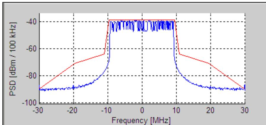
Figure 6-30. IQsignal 802.16e—PSD plot
