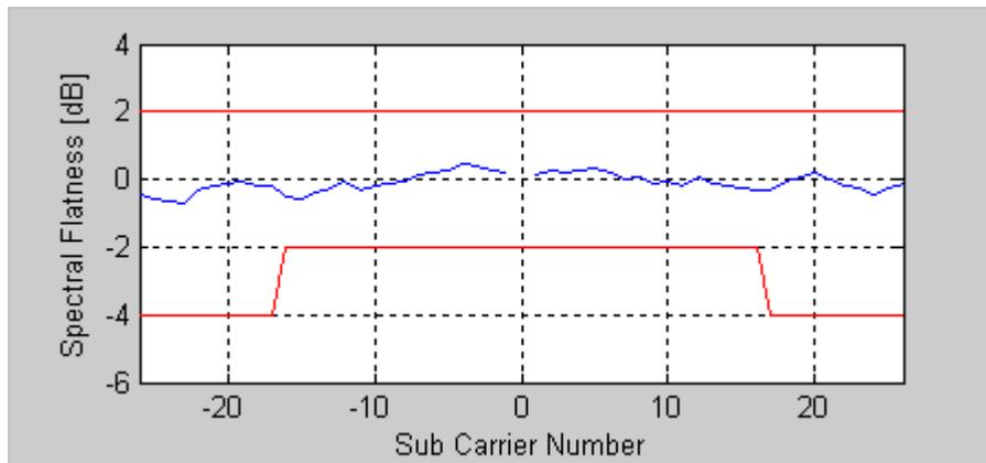
Figure 4-15. IQsignal 802.11a/g—Spectral Flatness Plot
