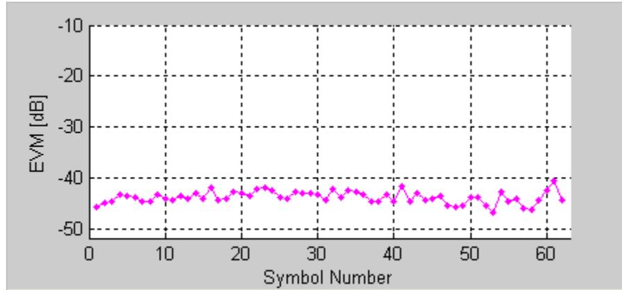
**Figure 6-5. IQsignal 802.16d—EVM vs. Symbol Plot**
