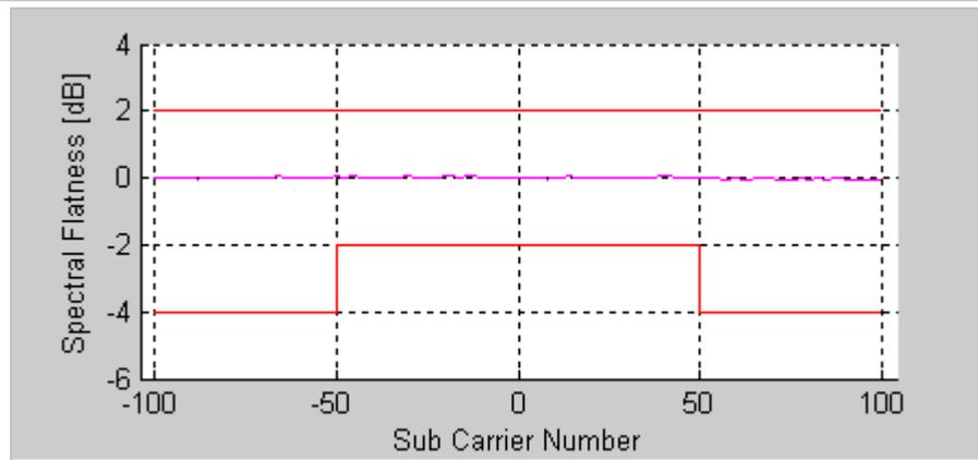
Figure 6-11. IQsignal 802.16d—Spectral Flatness Plot
