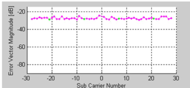
Figure 4-43. IQsignal 802.11n—EVM vs. Carrier
