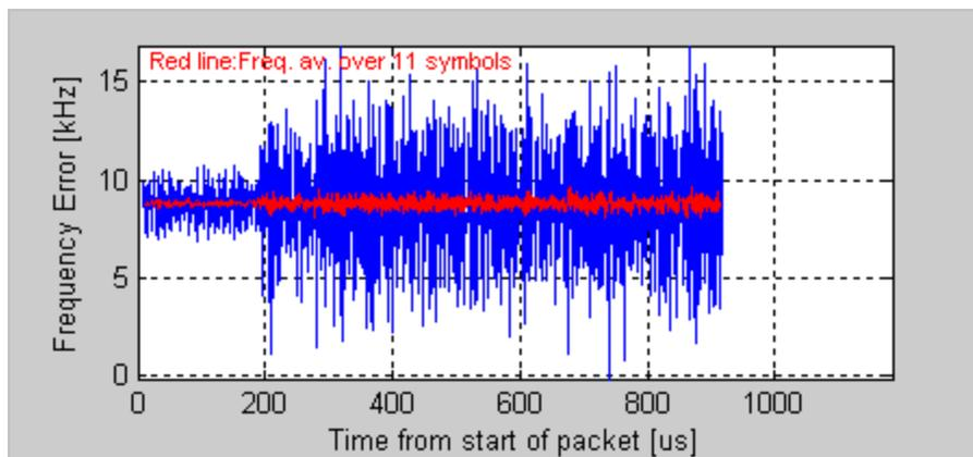
Figure 4-24. IQsignal 802.11b—Frequency Error Plot
