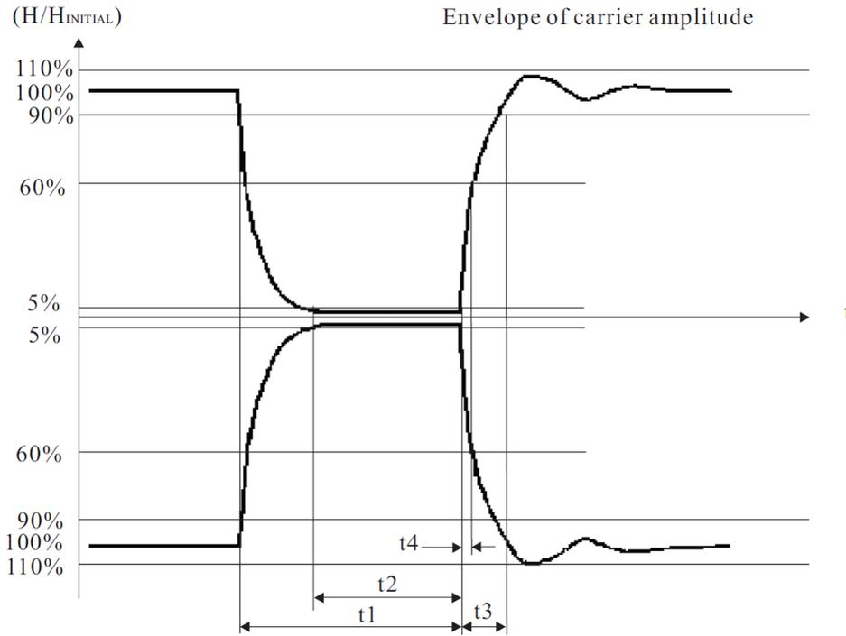
Figure 10-6. Pulse Shape for Miller coded ASK at 106kbps [Courtesy of ISO18092 (ECMA340) Specification]
