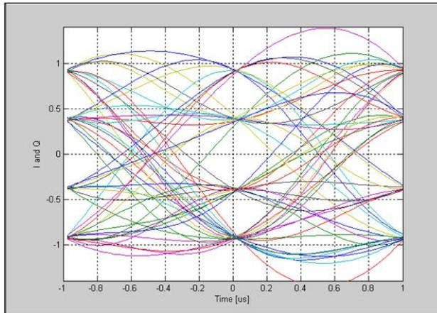
Figure 5-4. IQsignal Bluetooth—Eye Diagram Plot
