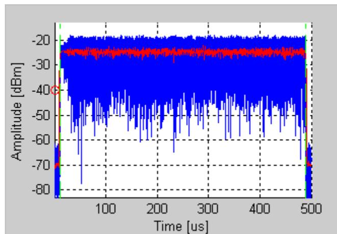
Figure 4-3. IQsignal 802.11a/g—Amplitude vs. Time
