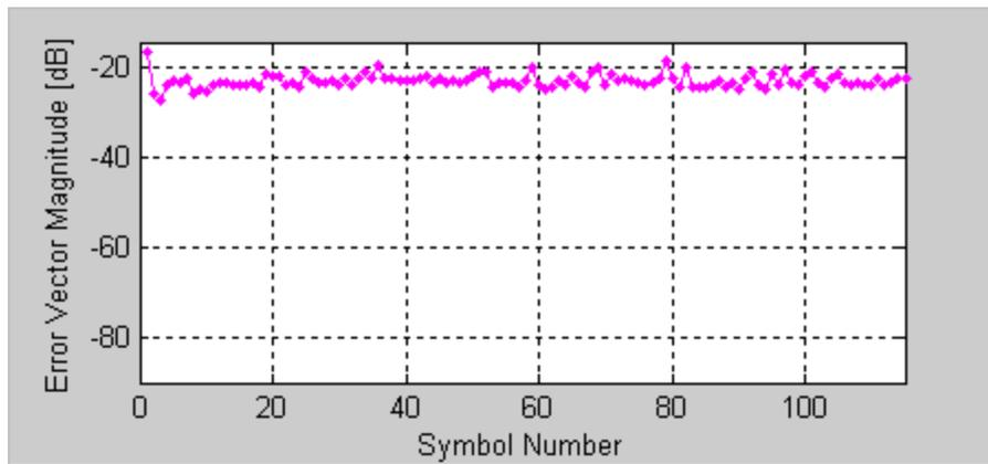
Figure 4-7. IQsignal 802.11a/g—EVM vs. Symbol
