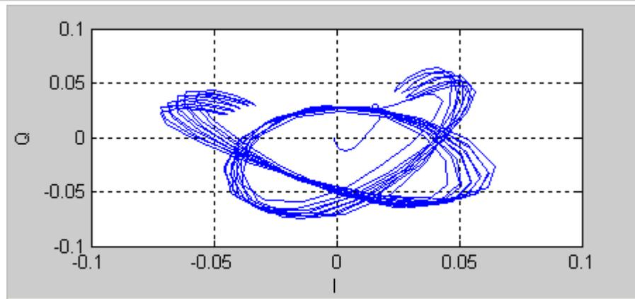
Figure 4-16. IQsignal 802.11a/g—STS Pretzel Plot
