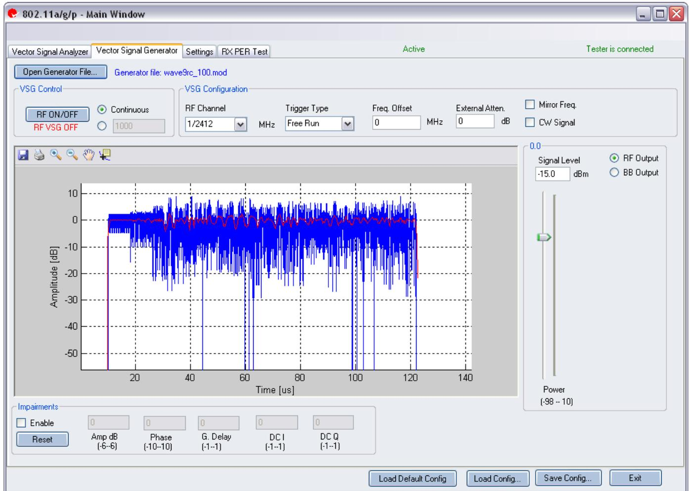
Figure 4-18. IQsignal 802.11a/g Application—VSG window
