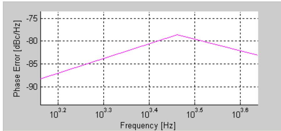
**Figure 6-25. IQsignal 802.16e—Phase Error (PSD) Plot**
