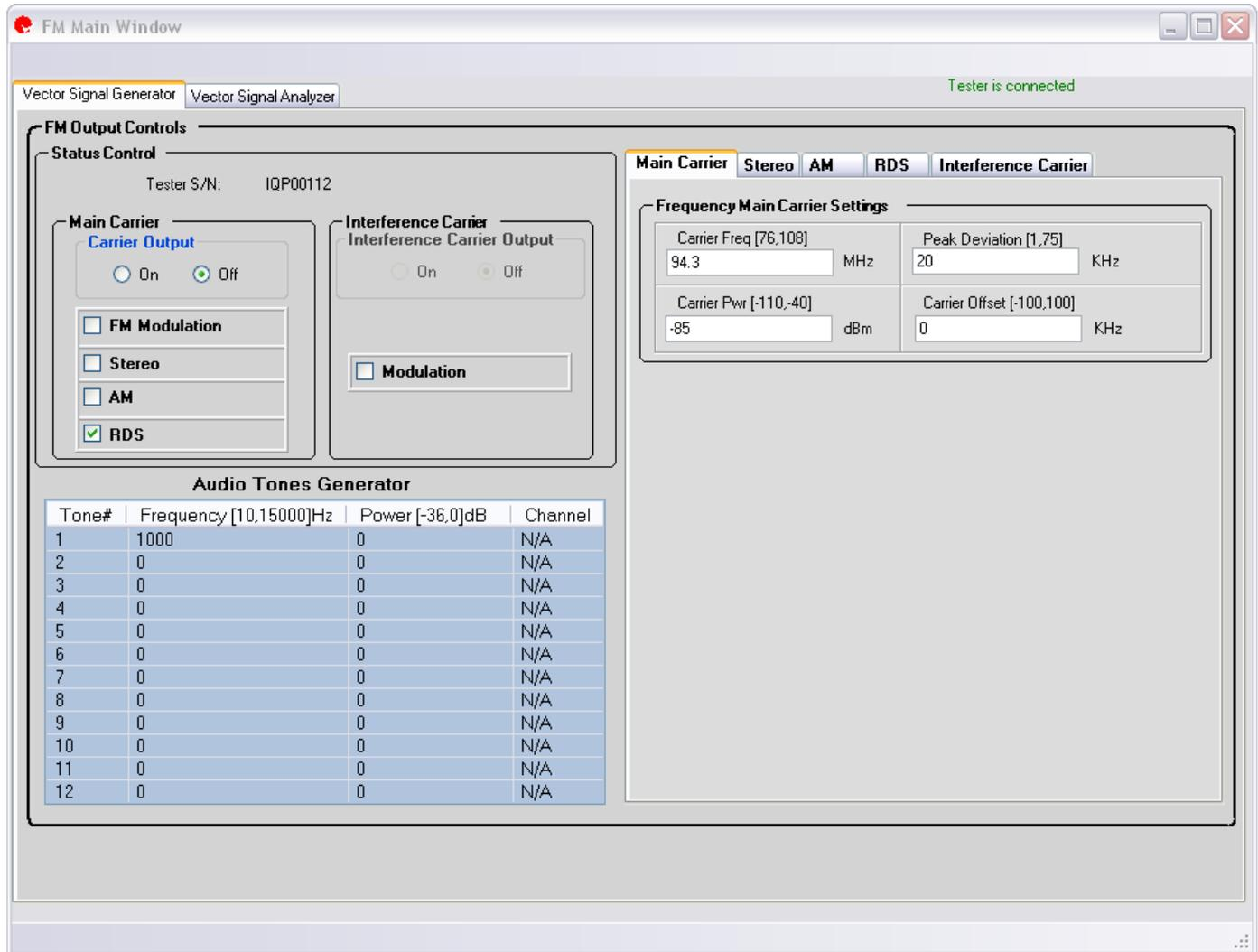
Figure 9-1. IQsignal—FM Main Window
