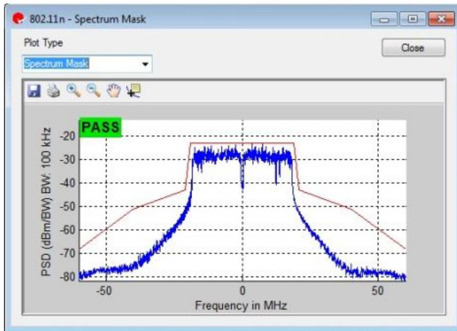
Figure 4-53. IQsignal 802.11n—Spectrum Mask at 120 MHz Frequency
