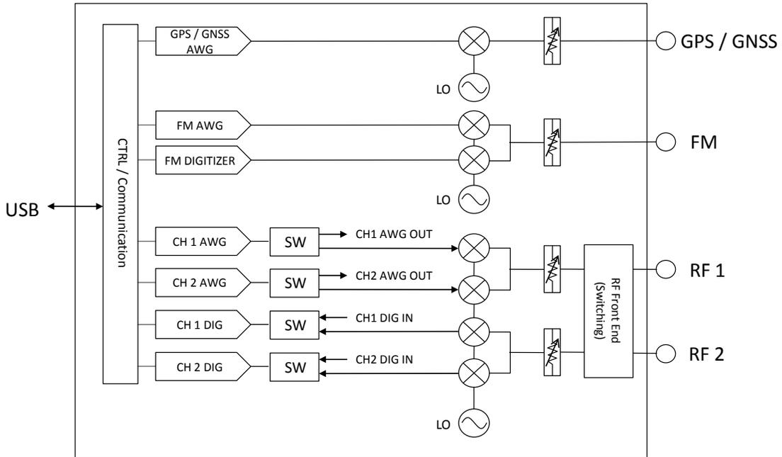
Figure 1-1. LitePoint IQ201X Test System—Basic Functional Block Diagram
