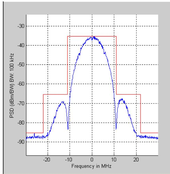
Figure 4-29. IQsignal 802.11b—PSD Plot
