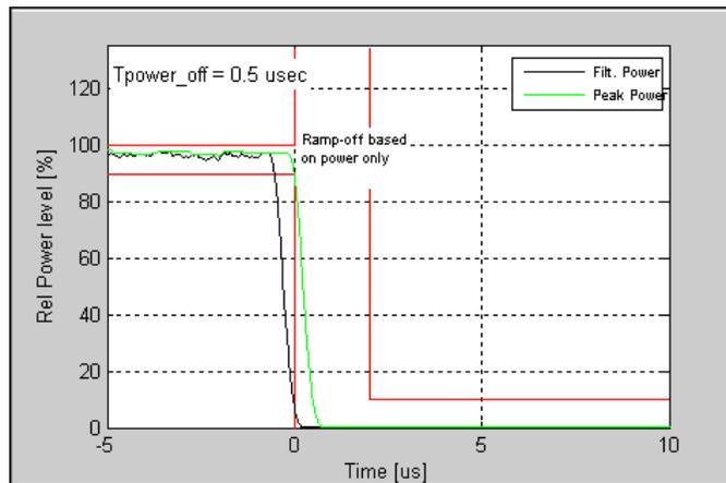
Figure 5-8. IQsignal Bluetooth—Power Down Ramp Plot
