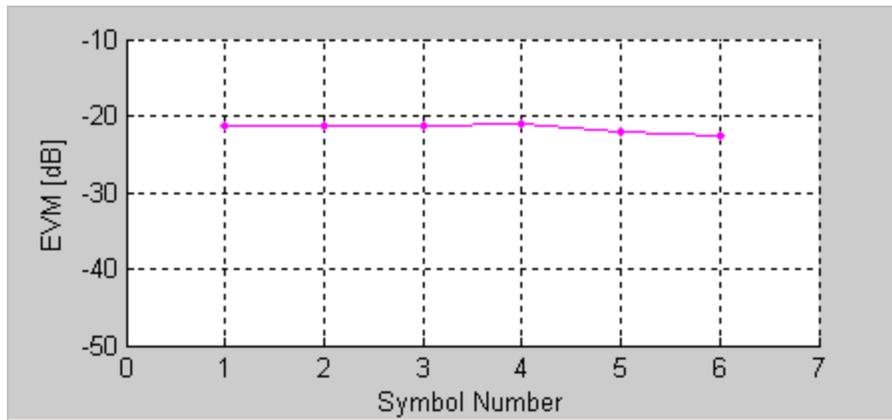
Figure 6-21. IQsignal 802.16e—EVM vs. Symbol
