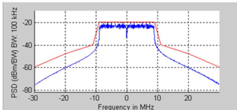
Figure 4-47. IQsignal 802.11n—Spectrum Mask
