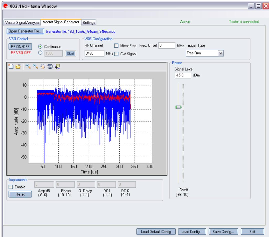
**Figure 6-15. IQsignal 802.16d Application—VSG Screen**
