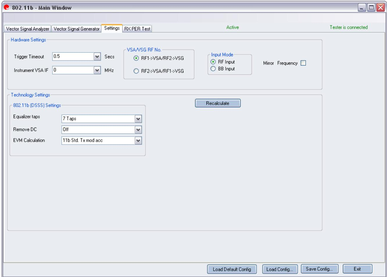
**Figure 4-34. IQsignal 802.11b—Settings Screen**
