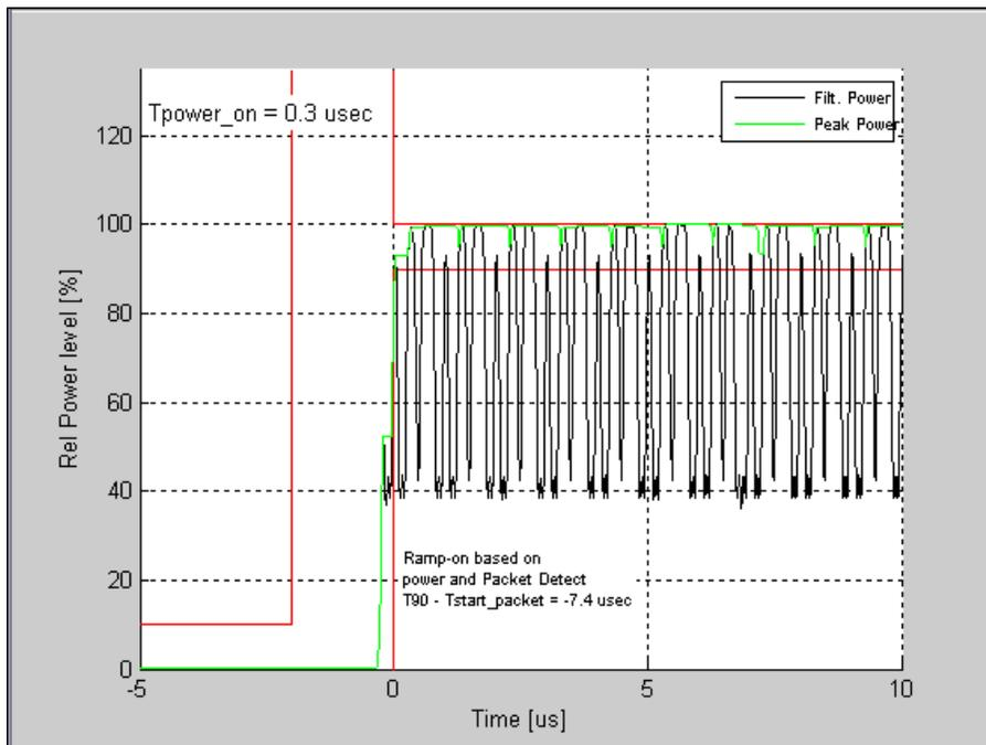
Figure 4-28. IQsignal 802.11b—Power On Ramp Plot
