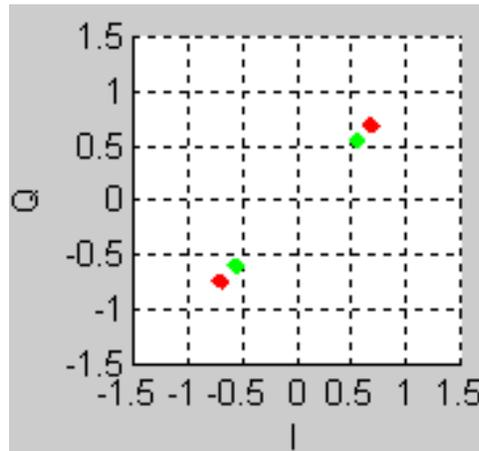
Figure 4-22. IQsignal 802.11b—Symbol Constellation Plot
