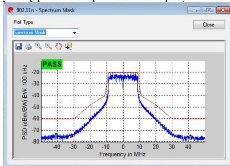
Figure 4-52. IQsignal 802.11n—Spectrum Mask at 100 MHz Frequency
