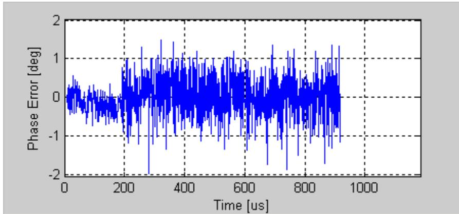
Figure 4-27. IQsignal 802.11b—Phase Error (Time) Plot
