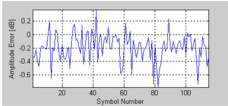
Figure 4-2. IQsignal 802.11a/g—Amplitude Error vs. Time
