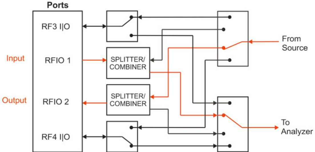
To use the RFIO 1 port as the input and the RFIO 2 port as the output, set up the RF Input using this menu setting or its equivalent command:
