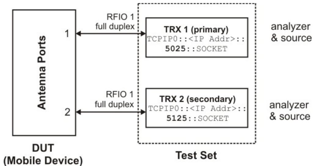
In the example setup shown here, TRX 1 runs the MIMO Modulation Analysis measurement, and is also configured to control TRX 2, which collects the second data stream. The primary TRX controls the measurement settings for the secondary TRX, and also processes the measurement data collected by the secondary. (The display window for the secondary will display a mostly-blank screen, with a message indicating that it is in use by the primary.)
