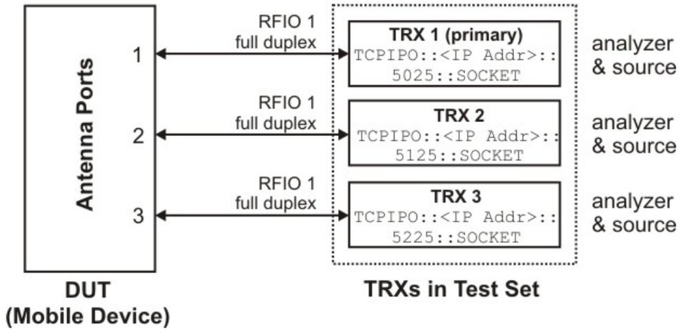
In the example setup shown here, TRX 1 runs the MIMO Modulation Analysis measurement, and is also configured to control TRX 2 and 3, which collect the second and third data streams.
