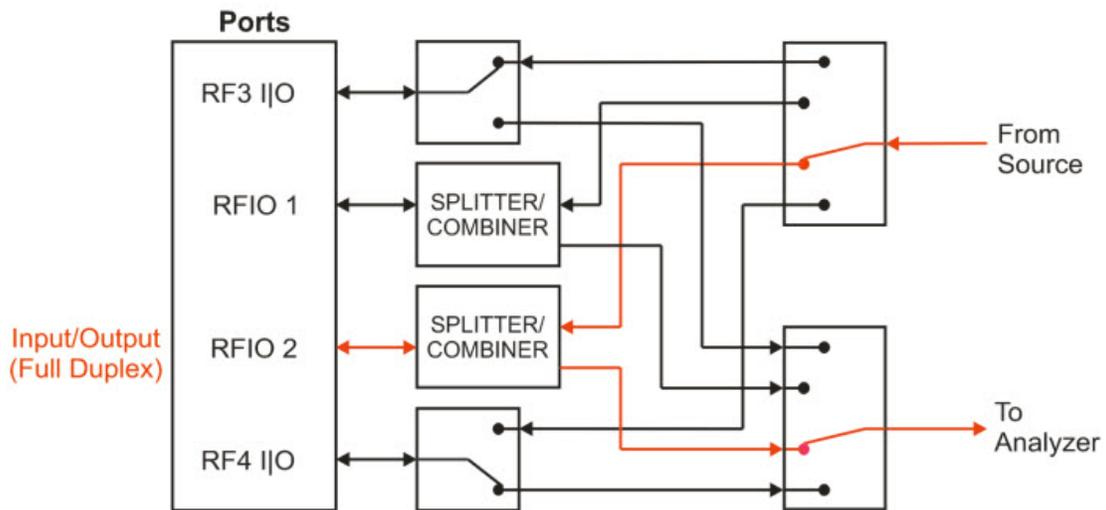
To use the RFIO 2 port as the input and output, set up the RF Input using this menu setting or its equivalent command:
