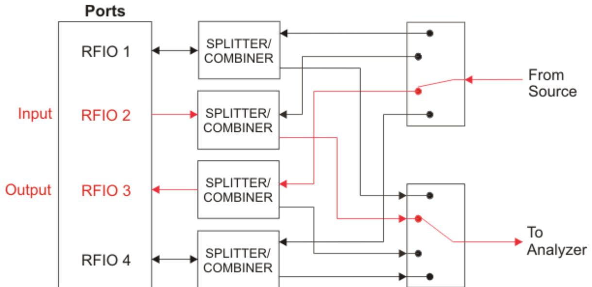
To use the RFIO 2 port as the input and the RFIO 3 port as the output, set up the RF Input using this menu setting or its equivalent command:
