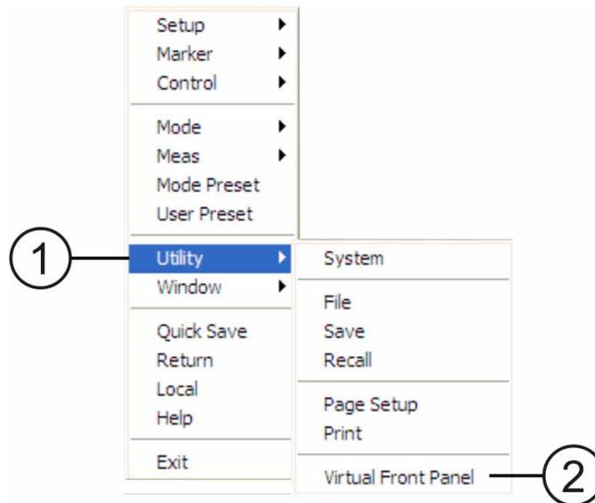
On the VFP the keys labeled "Key 1" through "Key 7" function as the menu keys. Using the mouse to click on a combination of the VFP keys and the menu keys on the display screen, you can operate the instrument as if it had conventional front-panel keys. The VFP frame shows "Left" or "Right" at the upper left corner of the frame, so that it's clear which sub-instrument within the PXI rack is being controlled by it.
