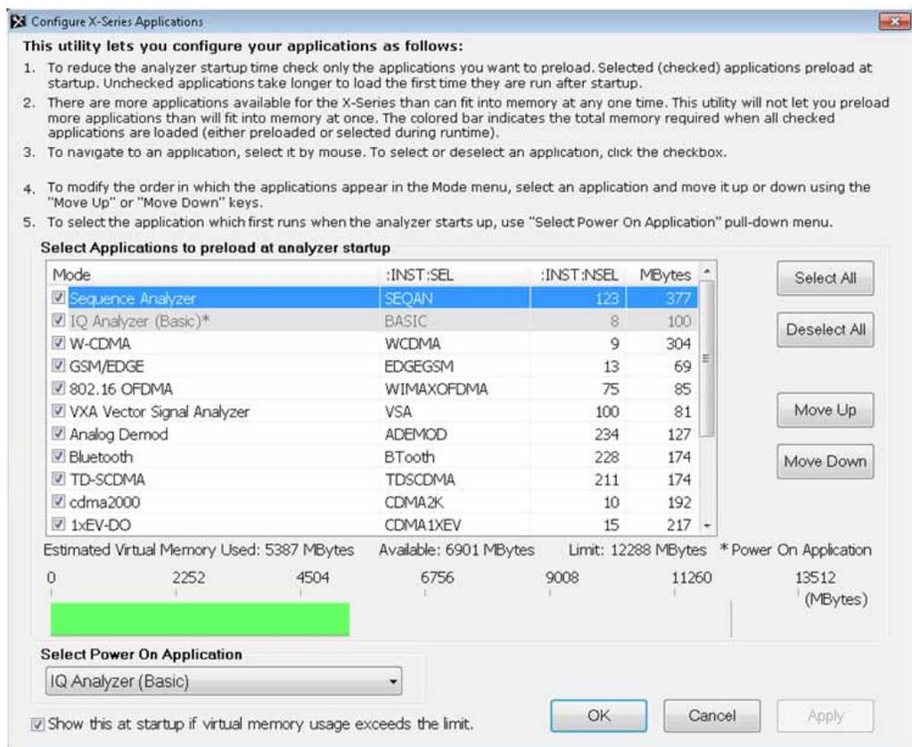
A selector at the lower left of the window allows you specify which application will be running when the E6640A starts up.
