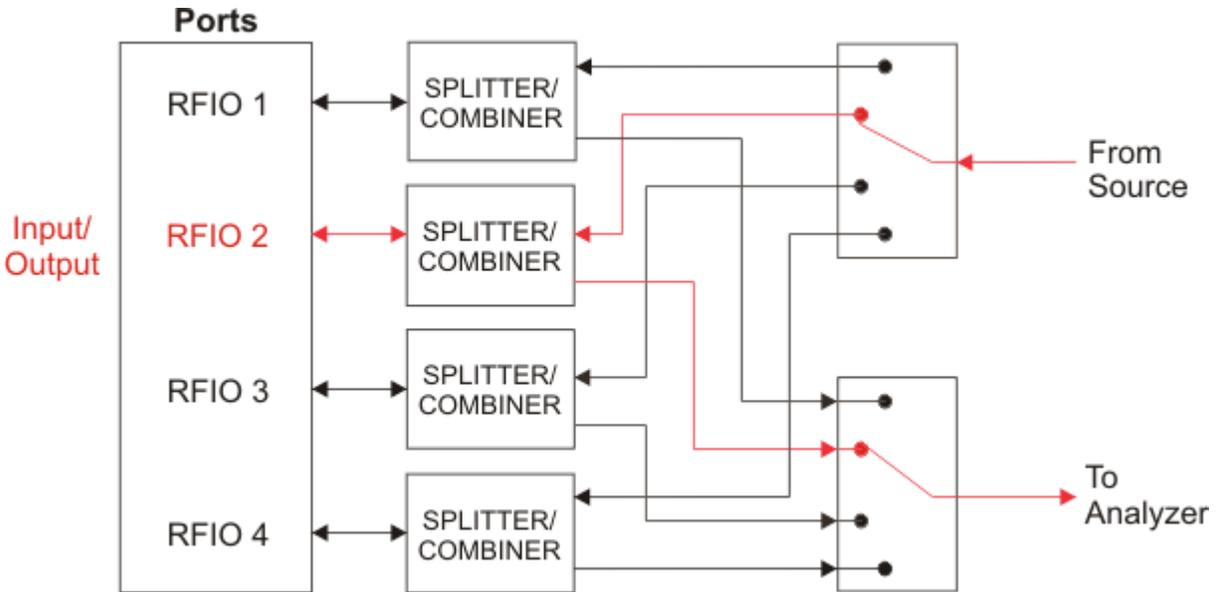
To use the RFIO 2 port as the input and output, set up the RF Input using this menu setting or its equivalent command:
