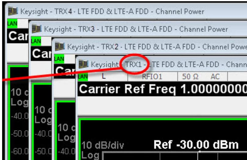
Although the test set as a whole is assigned only one IP address for the entire PXIe chassis, the individual TRXs within the chassis can be differentiated in network communication with the test set. The means of identifying a TRX depends upon the connection method, as outlined below.
