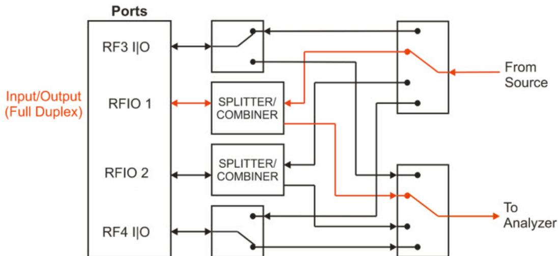
To use the RFIO 1 port as the input and output, set up the RF Input using this menu setting or its equivalent command:
