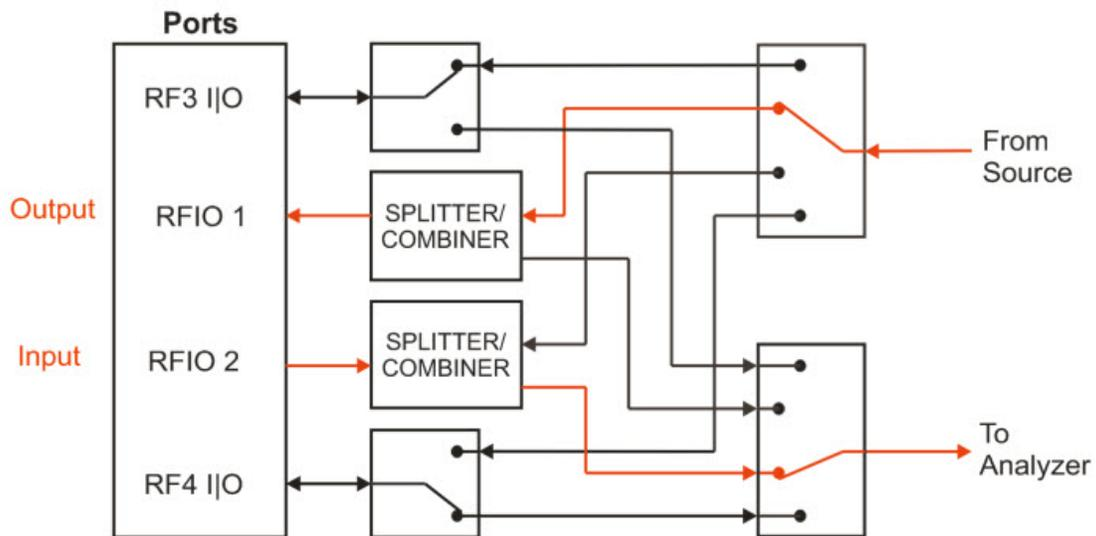
To use the RFIO 1 port as the input and the RFIO 2 port as the output, set up the RF Input using this menu setting or its equivalent command:
