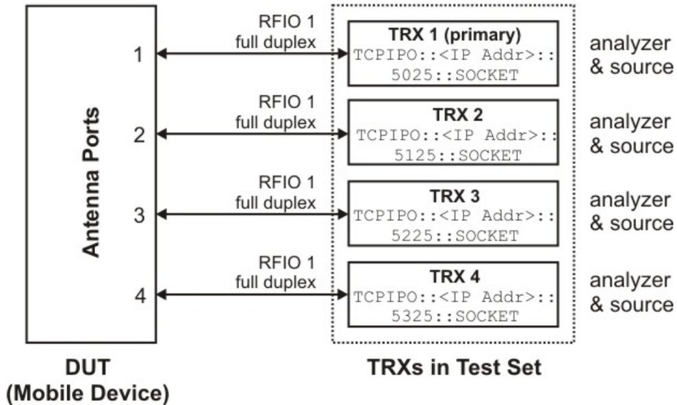
In the example setup shown here, TRX 1 runs the MIMO Modulation Analysis measurement, and is also configured to control TRX 2 to 4, which collect the second, third, and fourth data streams.
