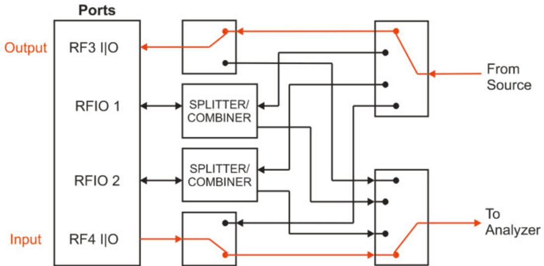
To define RF4 I/O as an input and RF3 I/O as an output, use the following steps.
