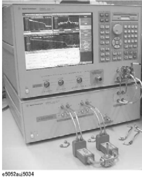
Figure 5-11 Setup for millimeter-wave phase-noise measurement with prescaler techniques
