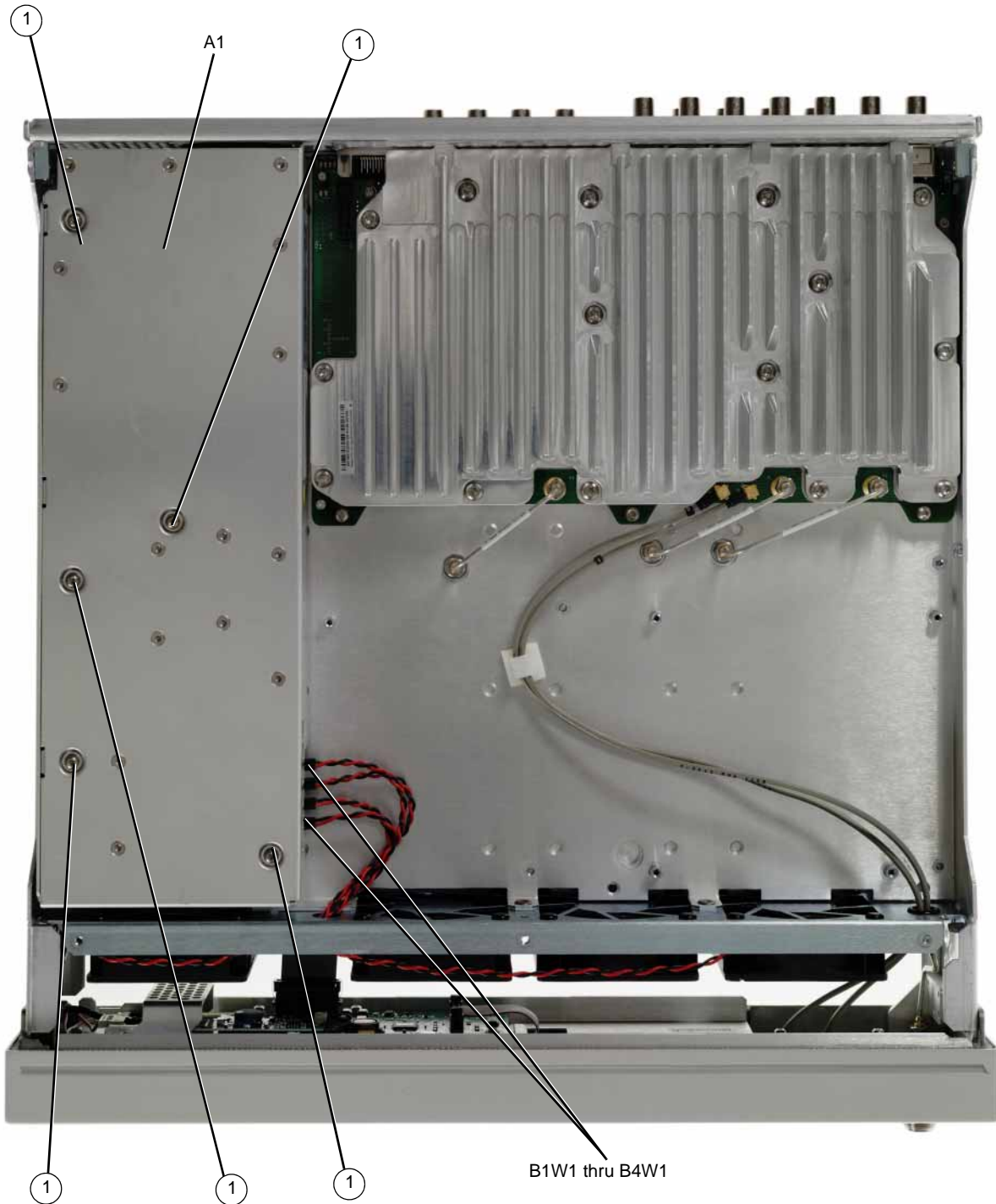
Figure 3-14 A1 Power Supply
